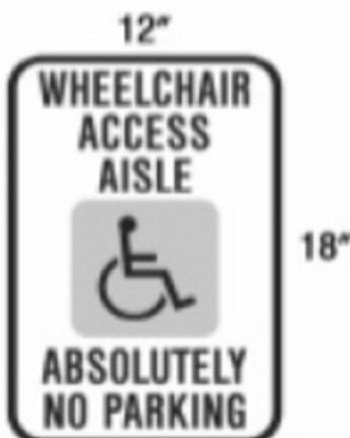
ACCESS AISLE SIGN
